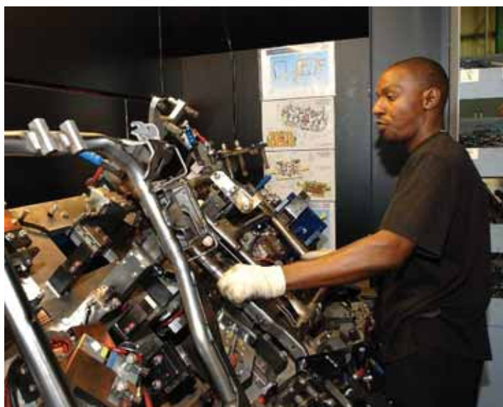
Honda Civic mig weld final assembly cell
